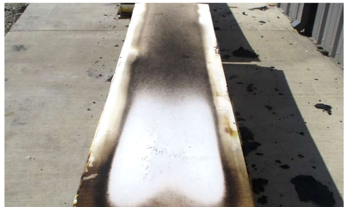
Fig.5. Charring and zero flame spread of MgO paneling following ASTM E2768 or extended ASTM E84 30-minute testing.
