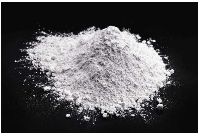
Fig.2. Calcined MgO originating from mined magnesite.
