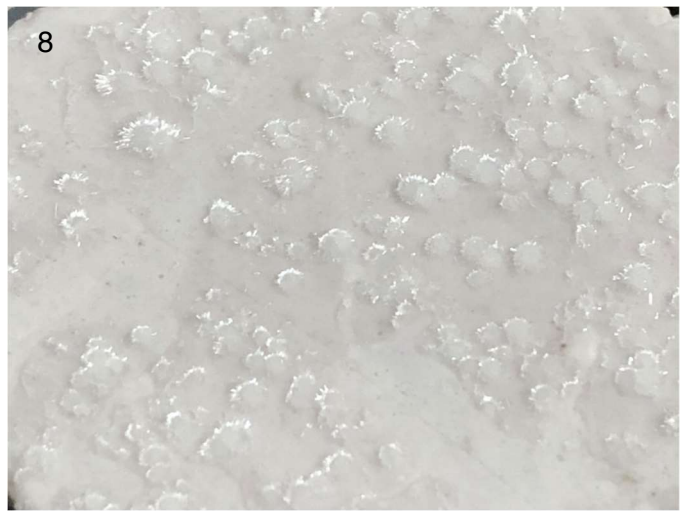
Figs. 7-8. Weeping of MgO panel at elevated relative humidity (Fig. 7). Salt crystals corresponding to evaporated weep droplets (Fig. 8).
