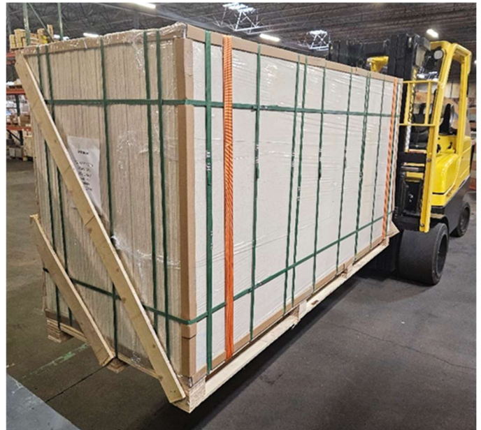
Fig.4. Palletized MgO showing panel edge orientation to accommodate oversea transport in shipping containers. Panels are typically re-palletized prior to distribution.
