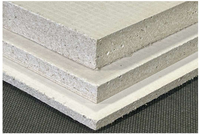
Fig.1. Magnesium oxide panels. Shown are three products with thicknesses ranging from 0.25” to 0.75”.
