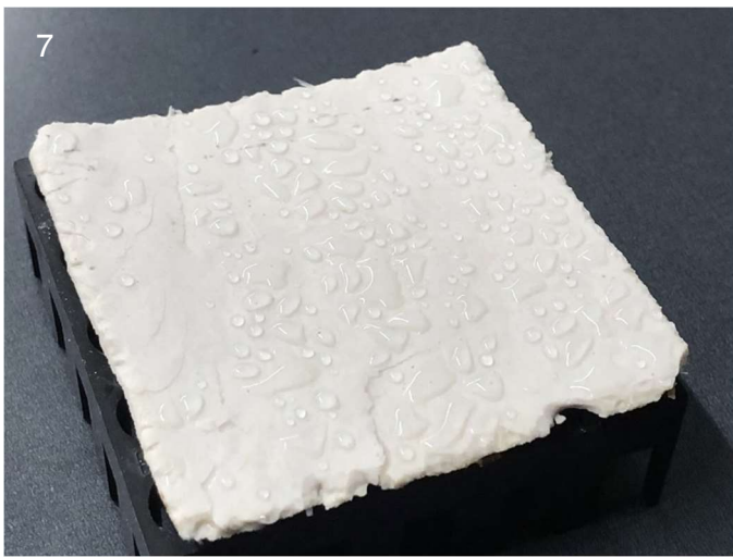
Figs. 7-8. Weeping of MgO panel at elevated relative humidity (Fig. 7). Salt crystals corresponding to evaporated weep droplets (Fig. 8).
