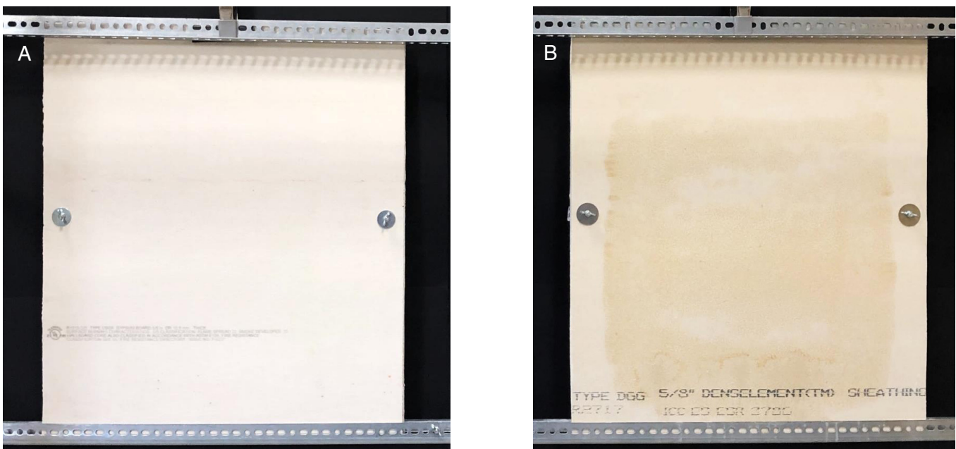
Fig. 3. Back side of Securock ExoAir 430 panel (A) and DensElement panel (B) following a seven-day face column test.
