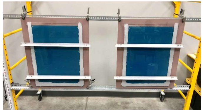
Fig.2. Established face columns at 21.6-inch fill height.
