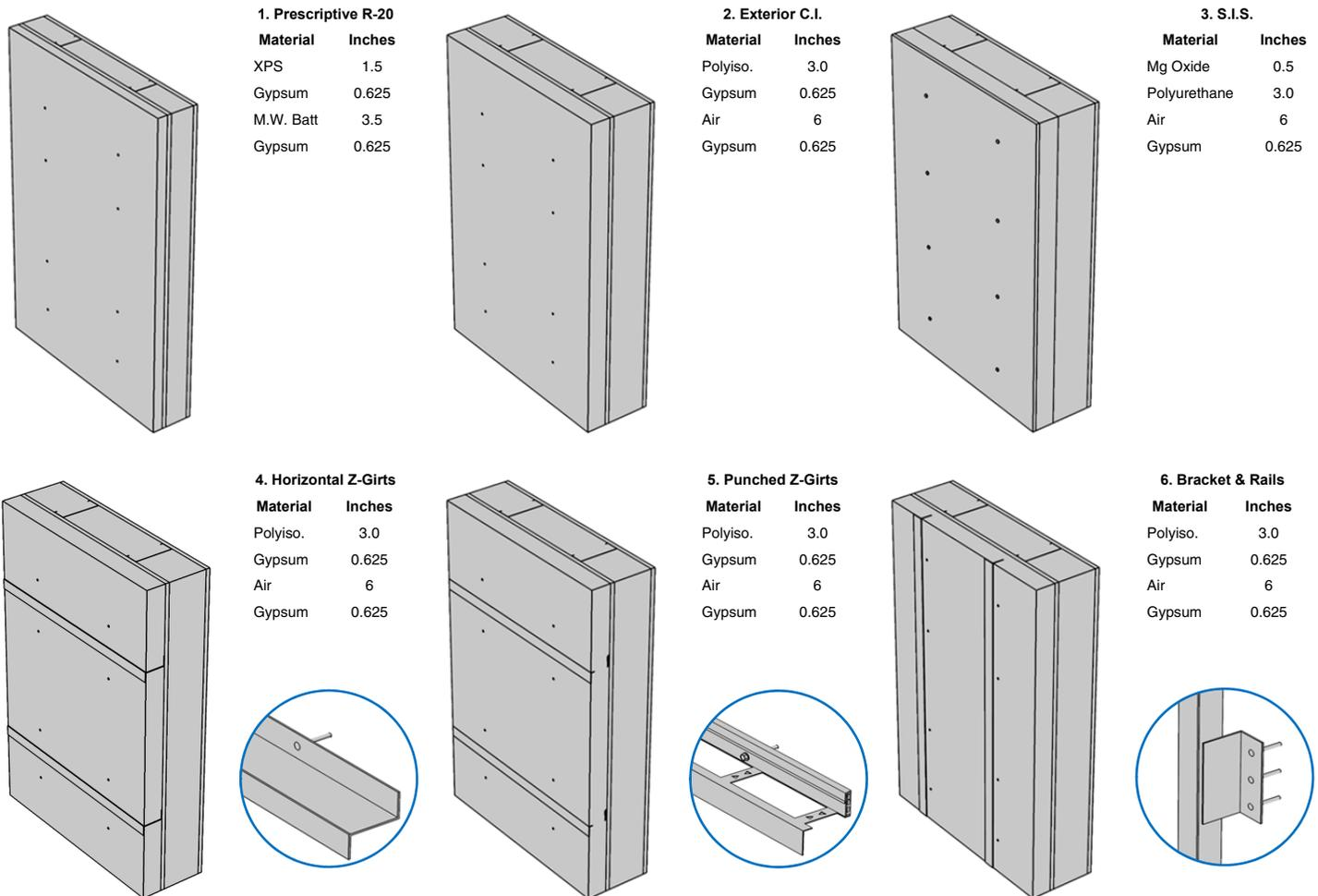
Fig. 1. Modeled wall assemblies. Geometries are shown with all corresponding components, including steel studs, fasteners, and cladding attachment systems.
