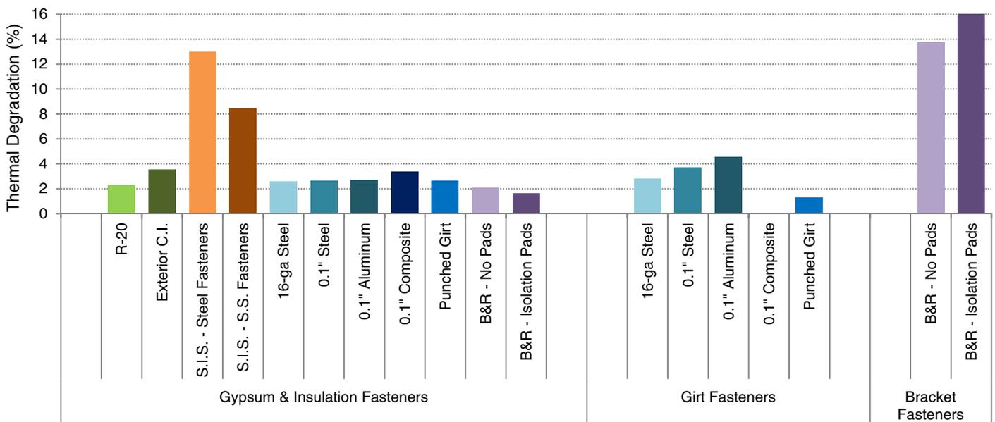
Fig. 6. The effects of fastener type on thermal degradation.
