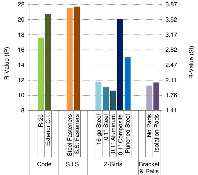
Fig.5. Total effective R-values of fully-configured assemblies.
