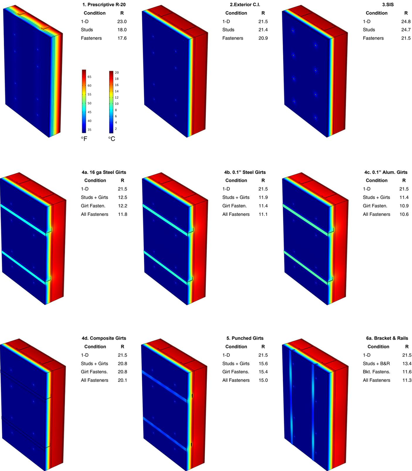
Fig. 4. Thermal performances of wall assemblies. Reported efficiencies represent walls configured with all components.
