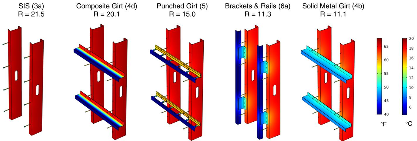
Fig. 3. Surface temperatures of primary bridging elements. Plots represent a common temperature range of 40-68 °F (4.4-20 °C). Total effective R-values represent all modeled components.
